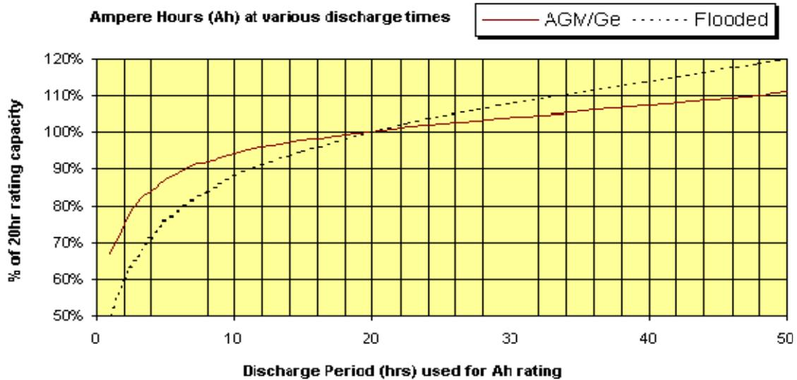
**Figure C1:** Battery efficiency at different draw-down rates.
