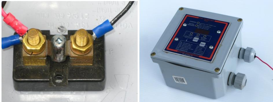
**Figure 3.1:** Amp meter shunt used to measure electrical current to and from the batteries (left). Battery meter logs data collected by an amp meter shunt (right)
