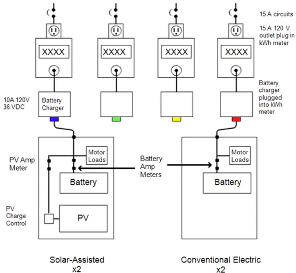
**Figure 3.2:** Monitoring set-up for evaluation of solar-assisted carts vs. conventional electric carts.
