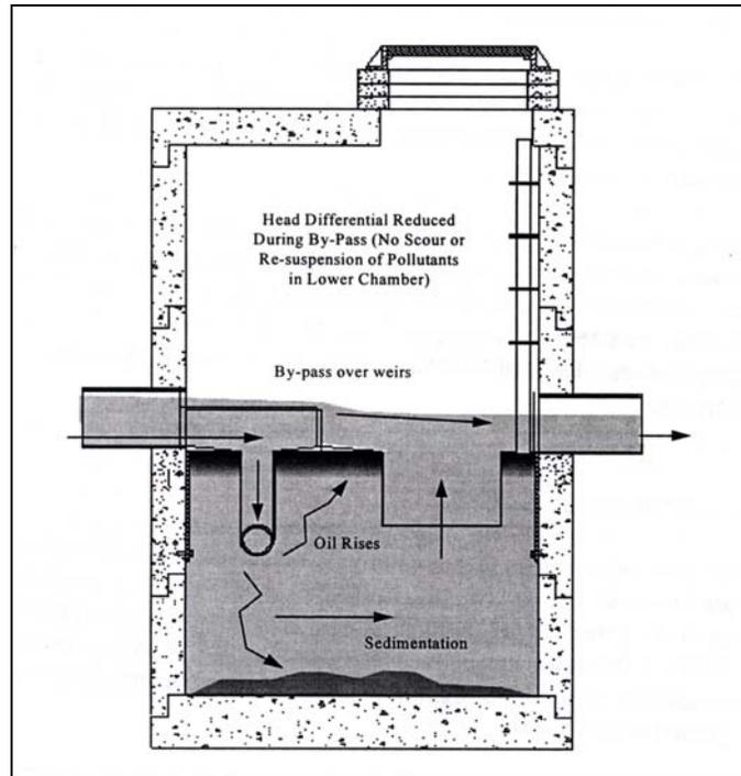
**Figure 2:** Stormceptor® operation during high flow conditions (Stormceptor®, 1996)
