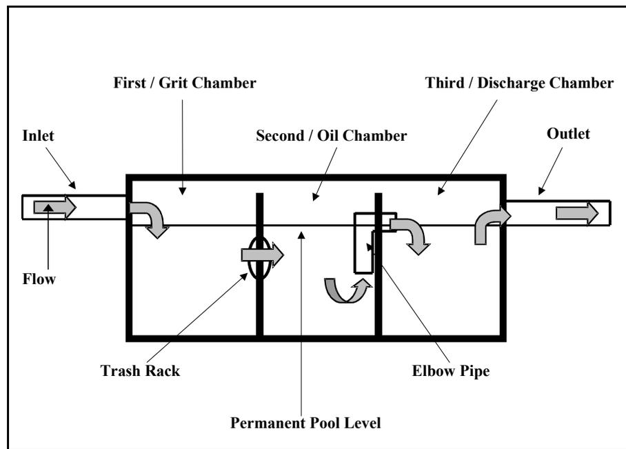
Figure 1 : Design of a three-chamber OGS
