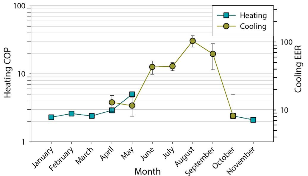
Figure 2. The monthly heating and cooling mode COPs for Earth Rangers. Cooling mode COPs are extremely good due to the primarily free-exchange mode of operation.
