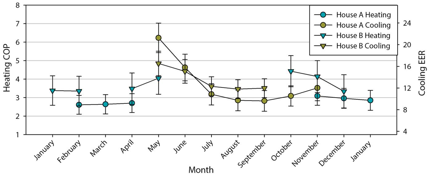
Figure 2. The monthly COP and EER from Peel House A and B.
