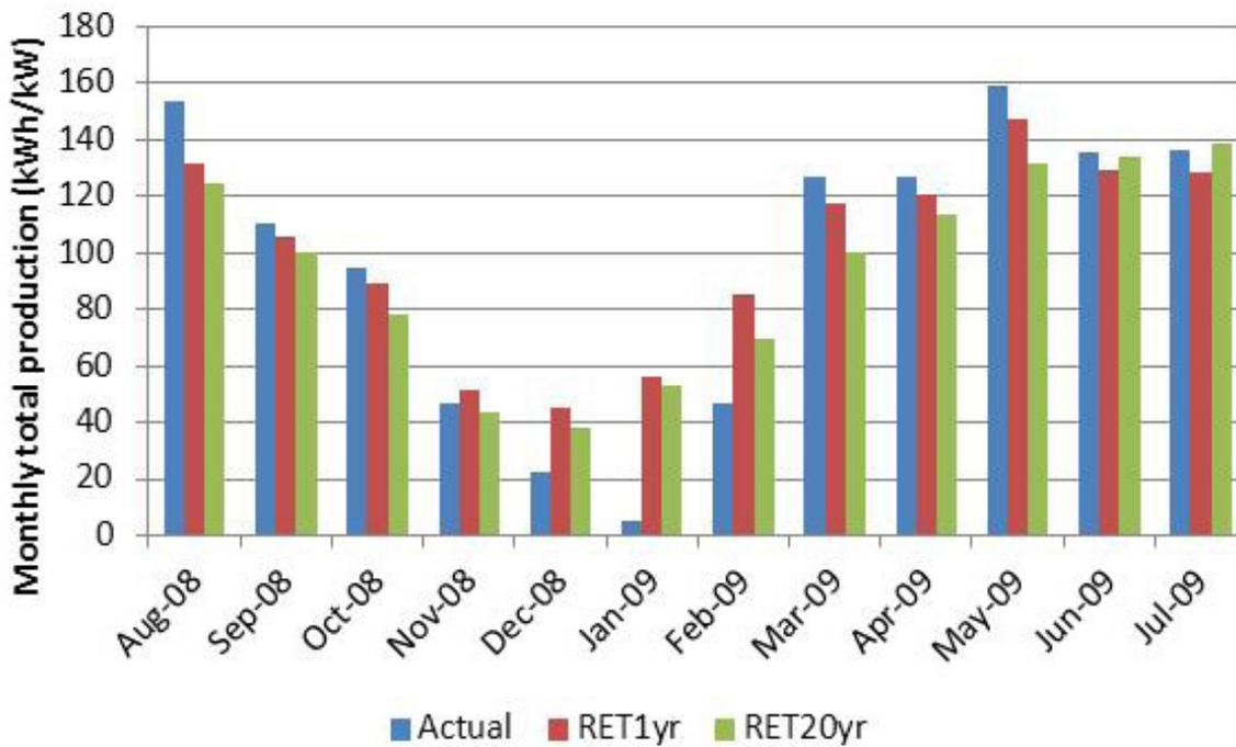
**Figure A4 (Figure 1).** Actual\* vs. RETScreen simulated performance (2008-2011 averages by month).
